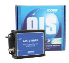
The AIS-2 Receivers are Dual Channel Parallel AIS Receivers with two AIS receivers monitoring both AIS channels at the same time and decoding both channels simultaneously. Unlike many AIS receivers that claim to be dual channel the AIS-2 receivers are true parallel receivers, ensuring that you receive the most up to date positions and information of all vessels around you.
